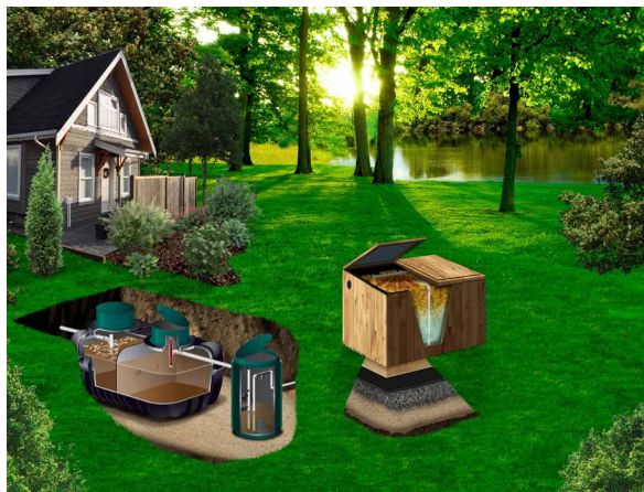
Waterloo Biofilter's anaerobic digester, Shed Biofilter, and disposal bed. Copyright: Waterloo Biofilter Systems Inc.
