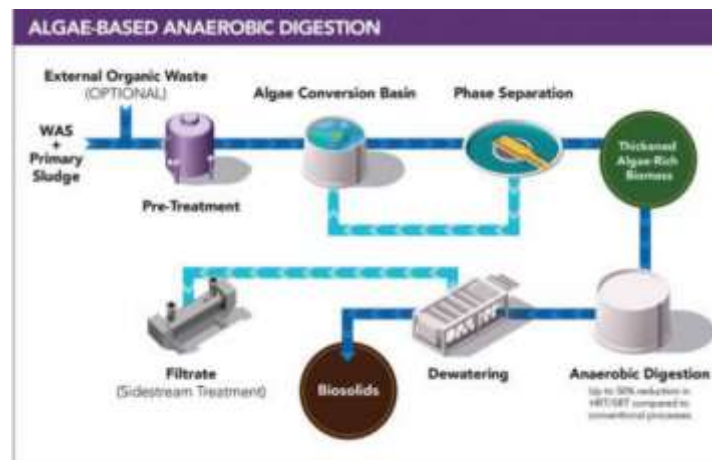
Figure B- 4. Schematic of BioAlgaNyx™ process
