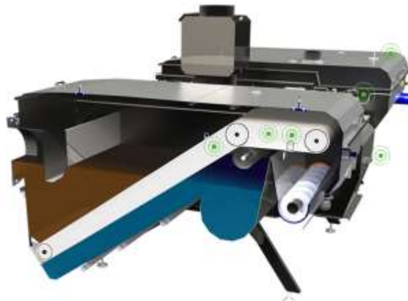
Figure B- 24.Schematic of Salsnes™ filter system
