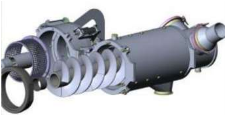
Figure B- 8. Schematic of Omnivore™ thickening system
