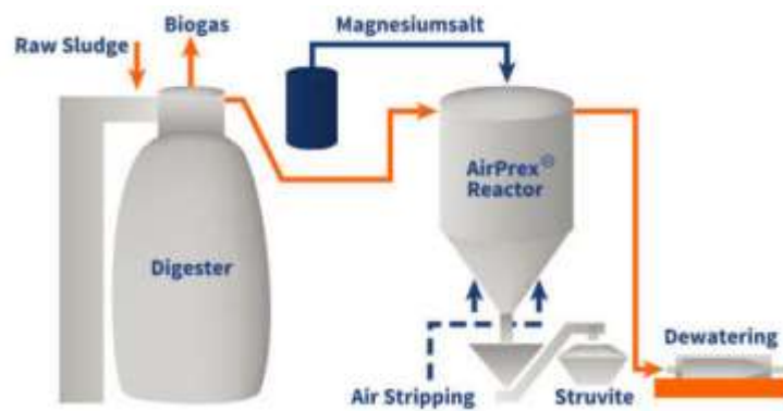
Figure B- 20. Schematic of AirPrex® system
