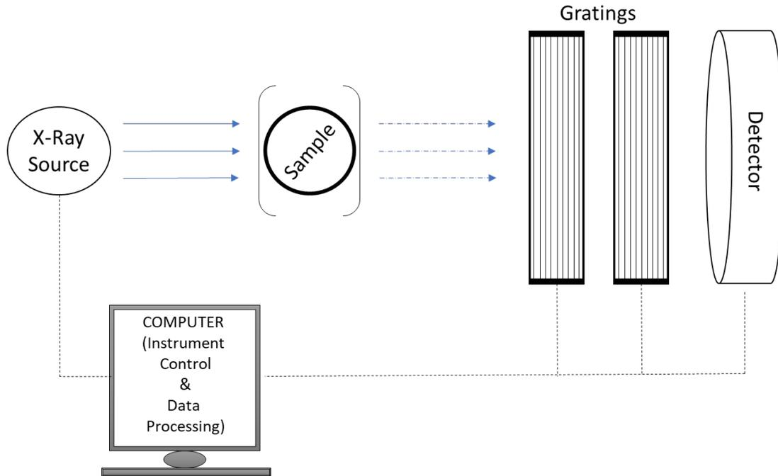
**Figure 10.** Schematic representation of X-ray imaging setup
