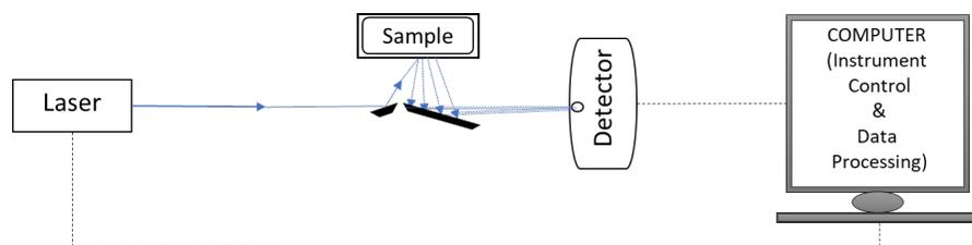
**Figure 11-b.** Schematic representation of Raman Spectroscopy setup
