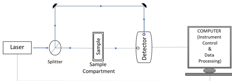
**Figure 11-a.** Schematic representation of FTIR Spectroscopy setup
