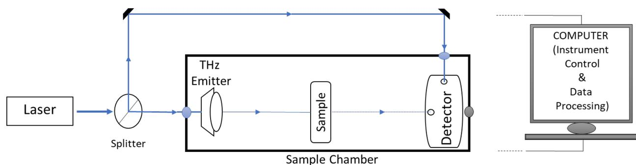
**Figure 9.** Schematic representation of THz imaging setup
