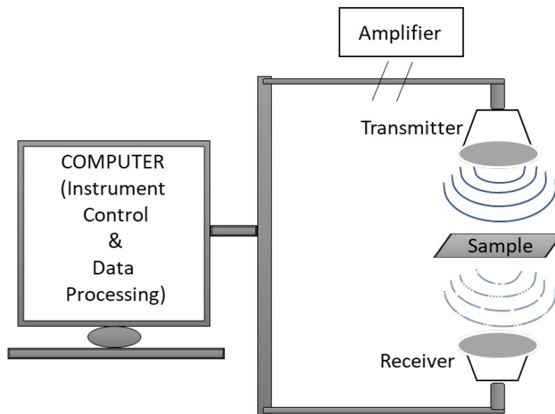
**Figure 8.** Schematic representation of ultrasound imaging setup
