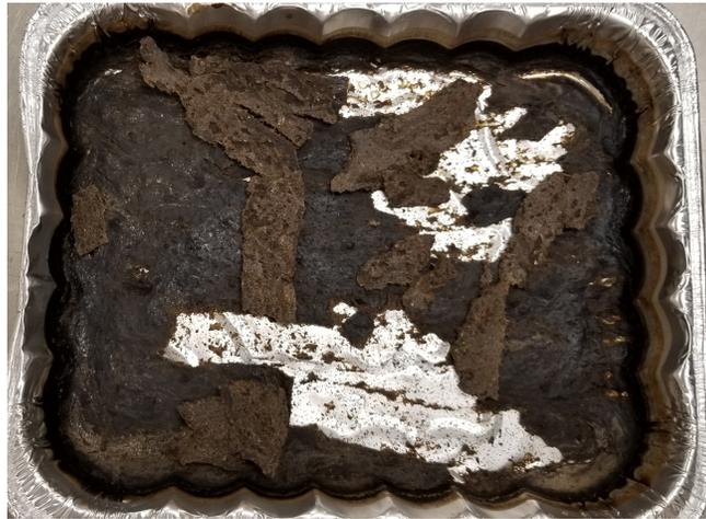
**Figure 3.** Trial 1. Sample C1 dried after three days in an oven at 50 °C and manually cracked.
