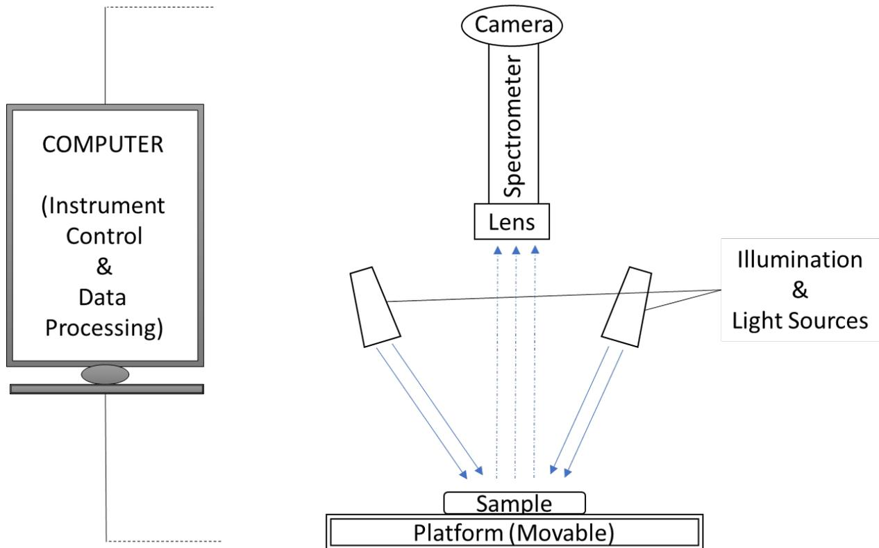
**Figure 6.** Schematic representation of HSI setup
