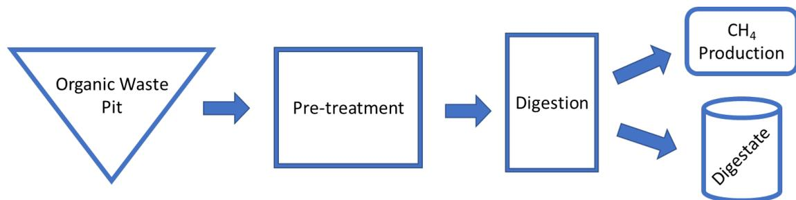
**Figure 1.** Schematic representation of processes employed in an AD facility
