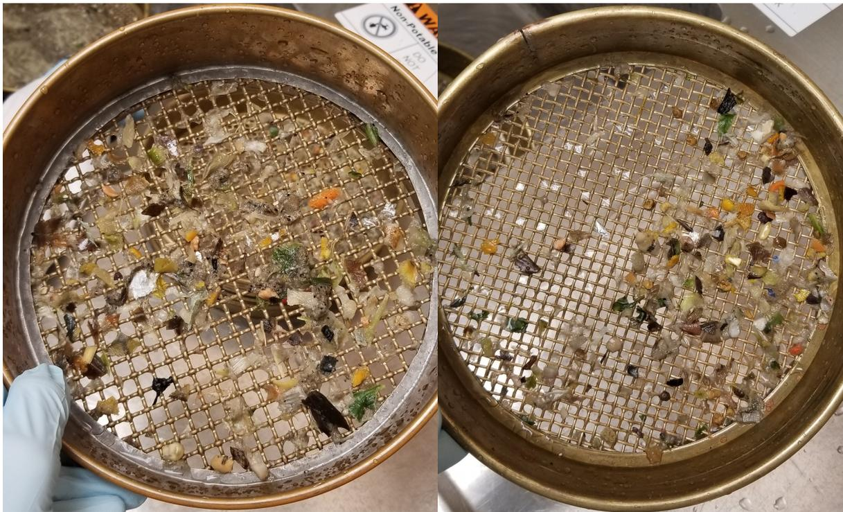
**Figure 4.** Trial 1. Left: Sample B1 6.73 mm sieve after rinsing. Right: Sample B1 4.0 mm sieve after rinsing.
