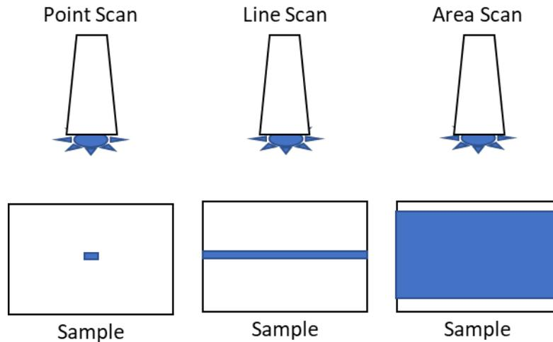
**Figure 7.** Different scanning options in HSI
